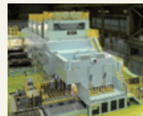
SMX-D Series large 5,700-ton servo tandem line
